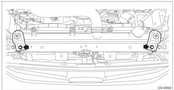
17) Remove the radiator from vehicle.
