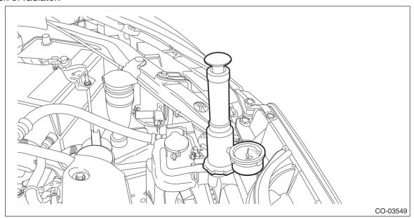
4) Apply a pressure of 157 kPa (1.6 kg/cm<sup>2</sup>, 23 psi) to the radiator, and check the following items.
